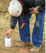
Careful installation of the vibration-detecting sensor before the survey begins is essential to data collection and analysis. The sensors will stay in place throughout the entire survey.
