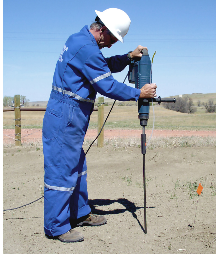
Soil gas is collected with a probe driven into the ground 3.5 feet during each sampling event.
