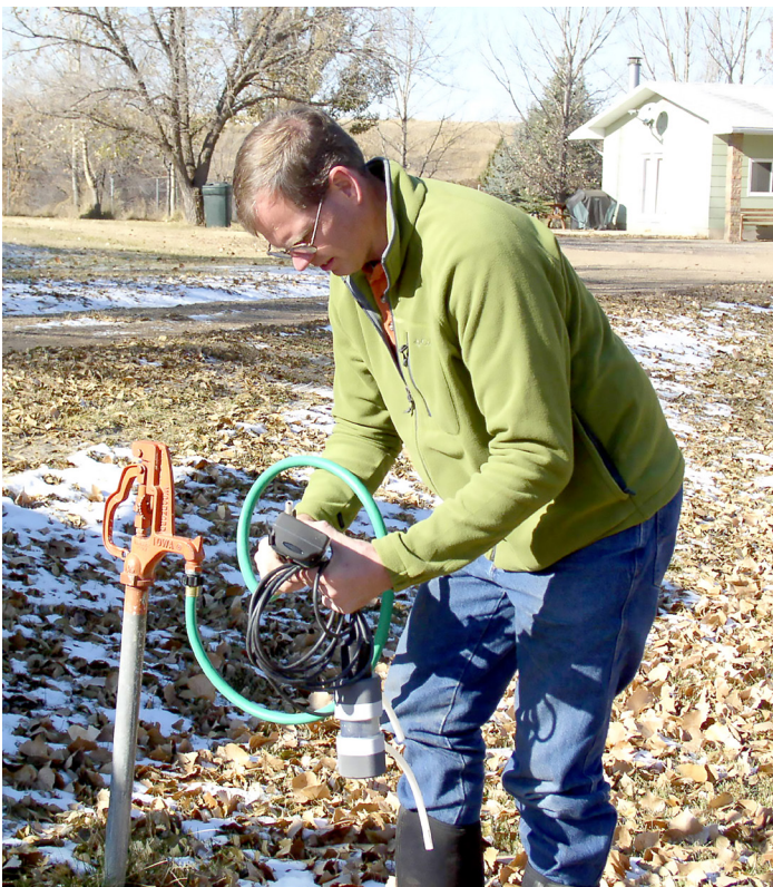
Technicians take some water measurements onsite before collecting groundwater to be analyzed in the laboratory.
