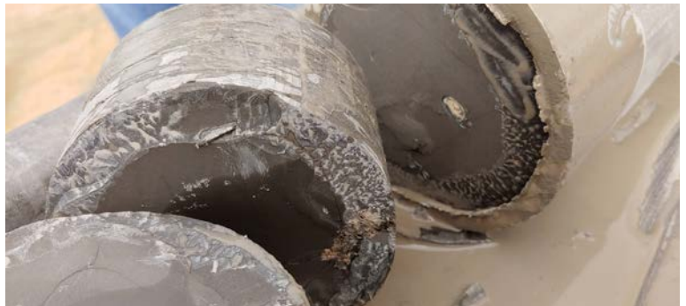
A closer look at core samples from more than 7000 feet below the surface: this shale is an example of a cap rock that will seal the CO 2 deep within the subsurface.
