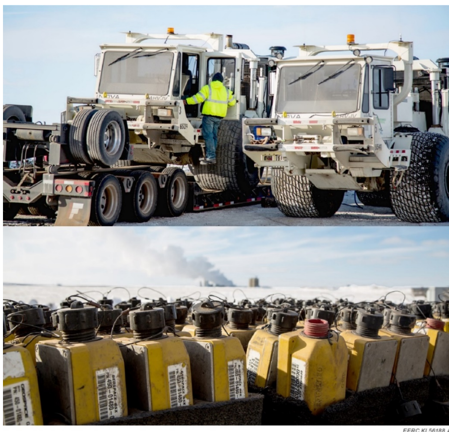
Figure 12. Vibroseis trucks from the RTE seismic survey (top) and seismic data loggers, with the RTE facility in the background (bottom).
