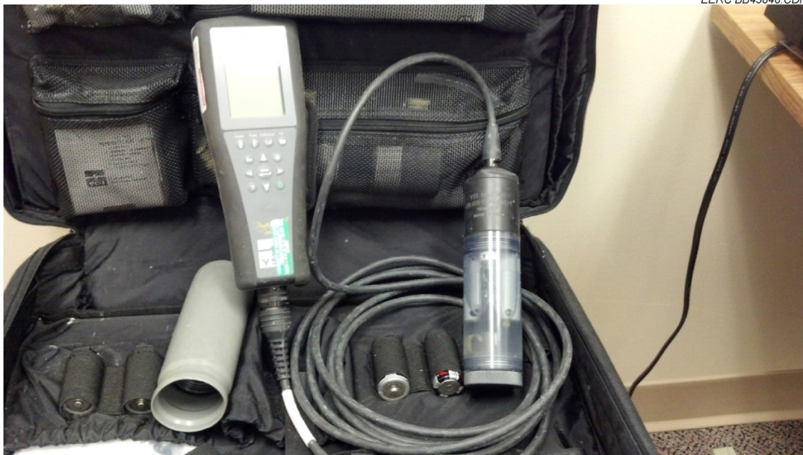
Figure B-1. YSI Professional Plus handheld multiparameter meter used for field measurement of water quality parameters.
