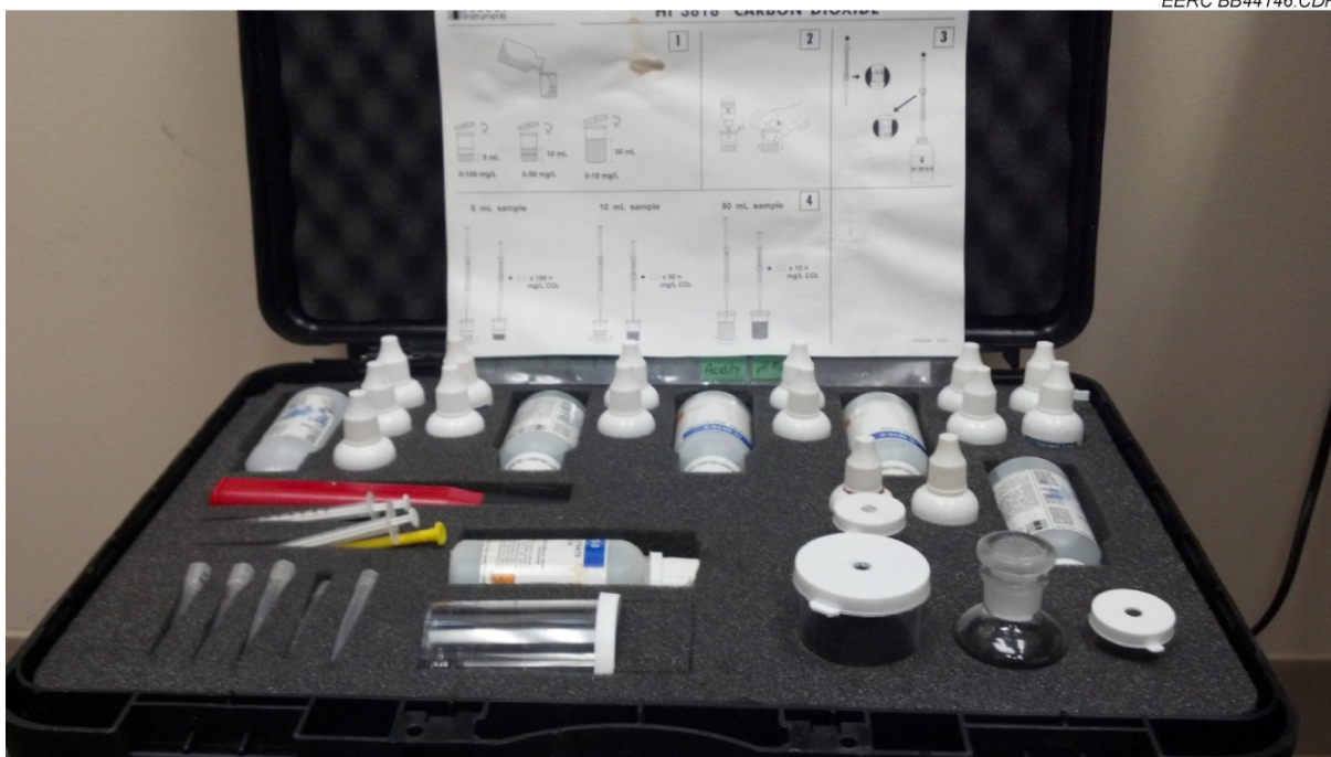
Figure B-2. Hanna field test kit for alkalinity as \text{CaCO}_3 , dissolved \text{CO}_2 , and chloride measurements.
