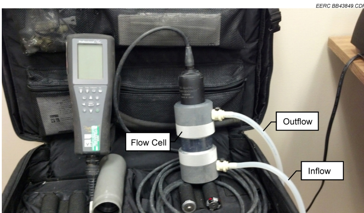
Figure B-3. YSI meter set up with flow cell application for measuring groundwater sample parameters.
