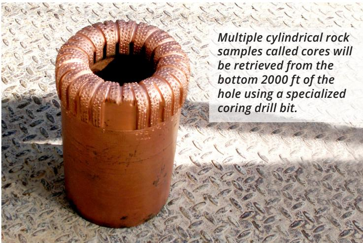
*Multiple cylindrical rock samples called cores will be retrieved from the bottom 2000 ft of the hole using a specialized coring drill bit.*
