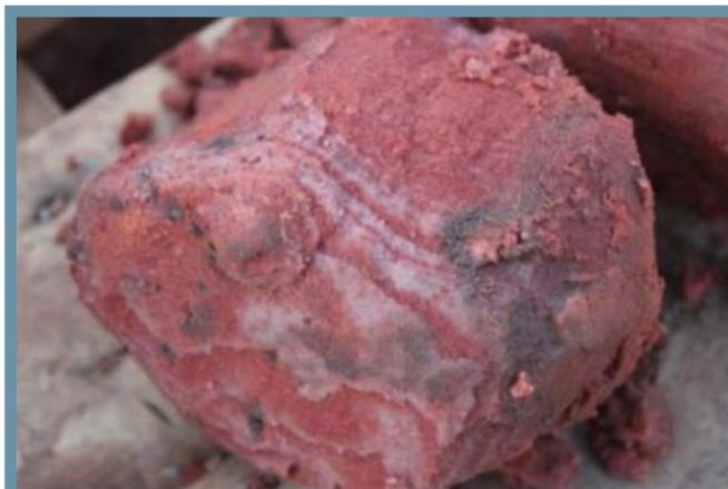
*A rock core cut from the target CO<sub>2</sub> storage layer 6400 feet below ground shows the pink sandstone of the Broom Creek Formation. It has the consistency of playground sand.*
