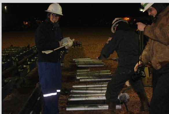
*Drilling exploratory holes allows researchers to collect rock samples deep below ground, cutting core that arrives at the surface encased in long metal sleeves. The sleeves are measured, labeled, and cut to 3-foot lengths for shipment to the lab.*
