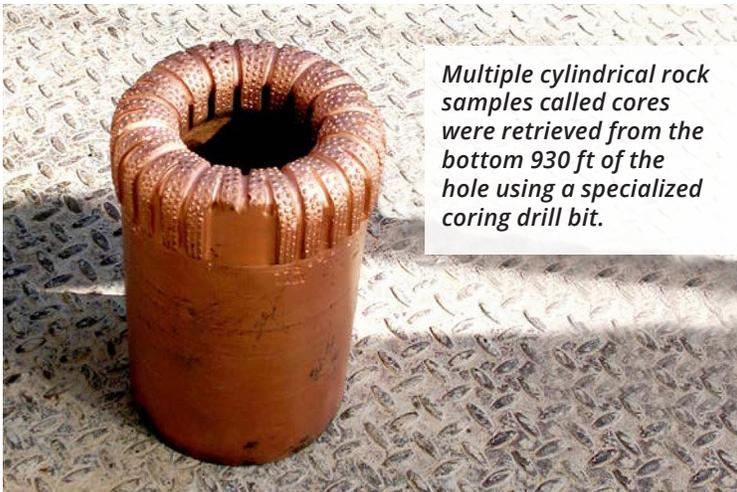
*Multiple cylindrical rock samples called cores were retrieved from the bottom 930 ft of the hole using a specialized coring drill bit.*
