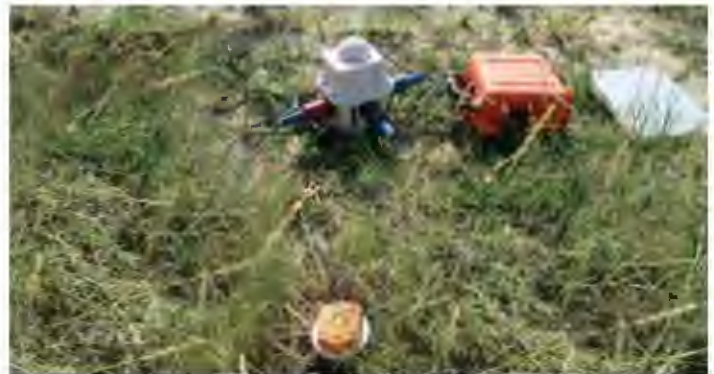
Example of a sensor location showing the sensor, battery pack, and Wi-Fi transmitter at a similar geophysical survey in Montana.
