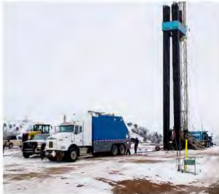
Wireline logging will collect data about the rock layers, their fluids, and their pressures.
